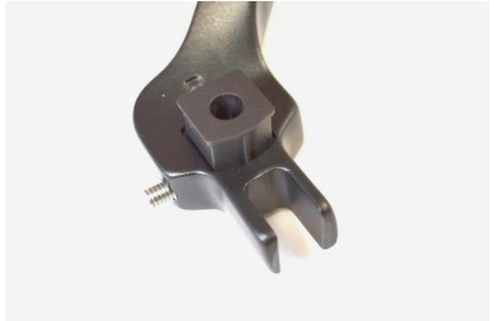
**STEP 4:** Now determine the best location of the handguard by moving it left or right to get the most coverage. The handguard should reach slightly beyond the end of the handlebars. **SEE PHOTO** Using 2 small spacers and 2 large spacers, position the handguard into the location you have chosen. **SEE PHOTO** Slide the long bolt through from the outside to the inside of the handguard and tighten with the lock nut. Position the handguard and now fully tighten the mounting bracket.
