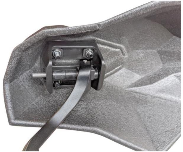
**At this time go back and check the torque of all fasteners. All fasteners may need to be retightened after the first ride. Check the tightness of the bracket and handguard before each ride.**
