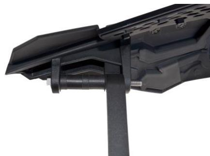
**STEP 7: At this time go back and check the torque of all fasteners. All fasteners may need to be retightened after the first ride.** Check the tightness of the bracket and handguard before each ride.
