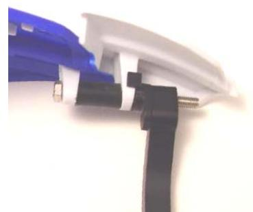
**Option 1 & 2 - RECOMMENDED:** The strongest mounting option is to have the bracket and no-spin spacer inside the handguard tabs. Thread the M6 x 45mm hex head bolt through the handguard tab, the no-spin spacer and bracket, and then the other tab. Thread the lock nut onto the bolt and tighten using 10mm wrenches.
