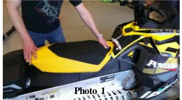
**Note:** Our seat riser kit can be installed over the OEM seat cover or if you prefer you can remove your OEM seat cover. To install over the OEM seat cover proceed to Step 3.
