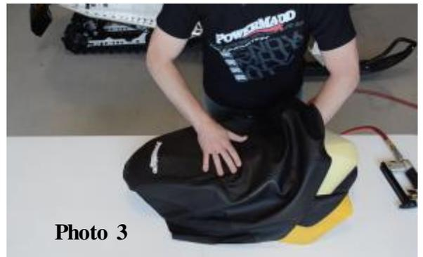
**Step 5:** Verify that the seams of the seat cover align with the seat foam and OEM seat. See photo 5.
