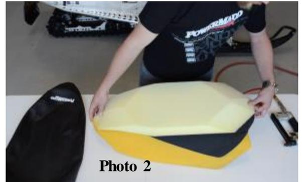
**Step 3:** Place the Seat Riser foam on the seat and center as shown in photo 2.
