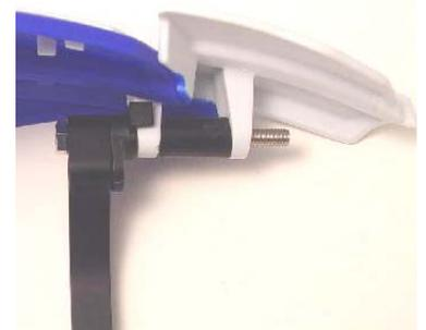
**Option 1 & 2 - RECOMMENDED:** The strongest mounting option is to have the bracket and no-spin spacer inside the handguard tabs. Thread the M6 x 45mm hex head bolt through the handguard tab, the no-spin spacer and bracket, and then the other tab. Thread the lock nut onto the bolt and tighten using 10mm wrenches.
