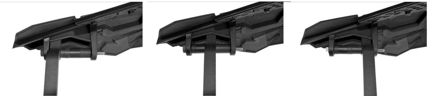
**STEP 5:** At this time go back and check the torque of all fasteners. All fasteners may need to be retightened after the first ride. Check the tightness of the bracket and handguard before each ride.
