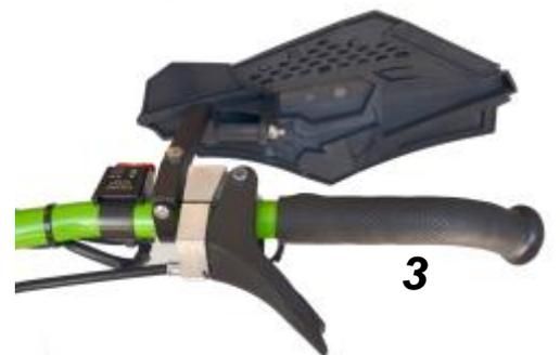
**STEP 3:** Insert the M6 x 25mm bolt with the flat washer through the bracket and the strap. Thread it into the square nut and tighten. This adjustment bolt is used to achieve the desired tightness of the mount. For now, leave the bracket loose so you can adjust the position up or down after attaching the handguard to the bracket.
