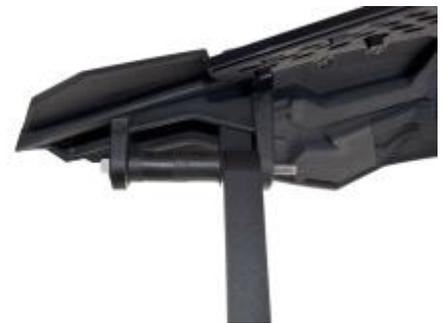
**STEP 5:** At this time go back and check the torque of all fasteners. All fasteners may need to be retightened after the first ride. Check the tightness of the bracket and handguard before each ride.
