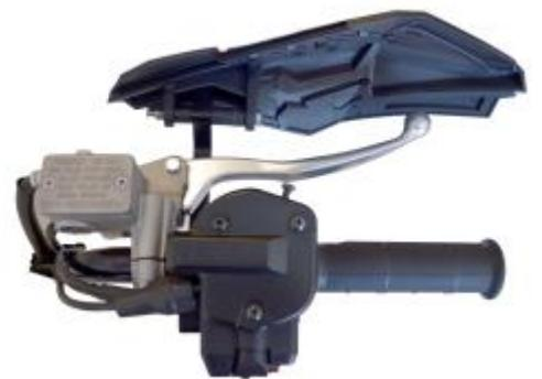
Bracket is positioned under the lever.
