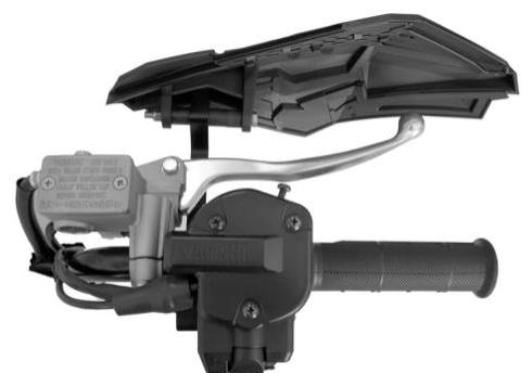
Bracket is positioned under the lever.
