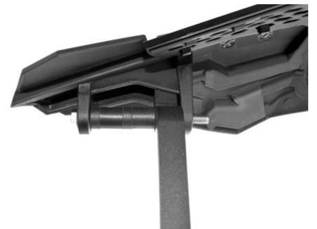
**STEP 7:** At this time go back and check the torque of all fasteners. All fasteners may need to be retightened after the first ride. Check the tightness of the bracket and handguard before each ride.
