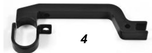
**STEP 4:** Slide the short steel strap onto the handlebars. Any wires should go outside the strap.
