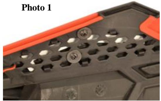
Route LED light wires along handlebar towards the steering stem. after you have completed all the steps secure the wires to the handle bars using the supplied cable ties. Note: Verify that no wires will be cut or pinched by any moving parts.
